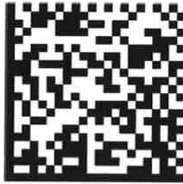
Figure 1. ECC200 data matrix symbol
