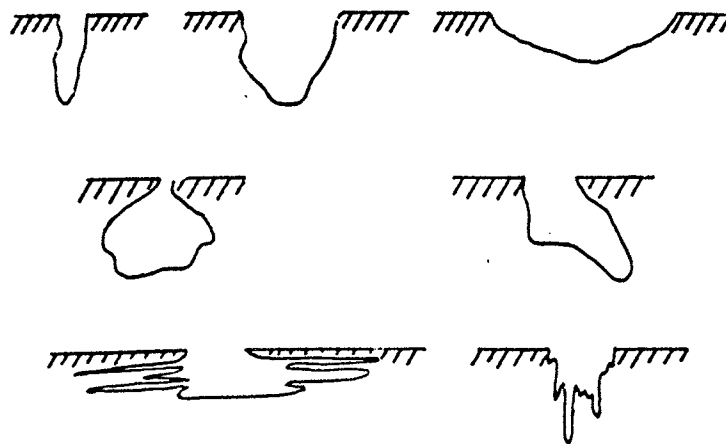
Fig. 2. : Various pit forms by pitting corrosion.
